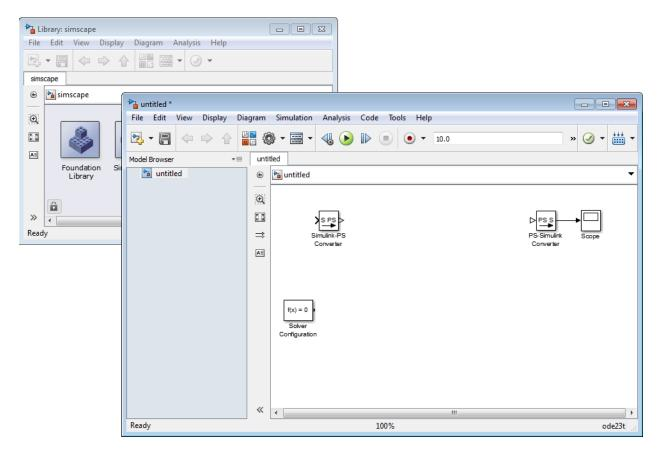
By default, the model name is not specified, the model contains a Solver Configuration block with the default solver set to ode23t, a Simulink-PS Converter block, and a PS-Simulink Converter block connected to a Scope block.
